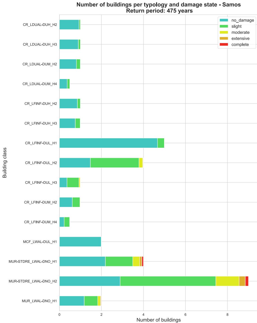
Figure 85. Number of school buildings per GEM typology and damage state in the city of Samos for PSHA scenario with T_m=475 yrs.
