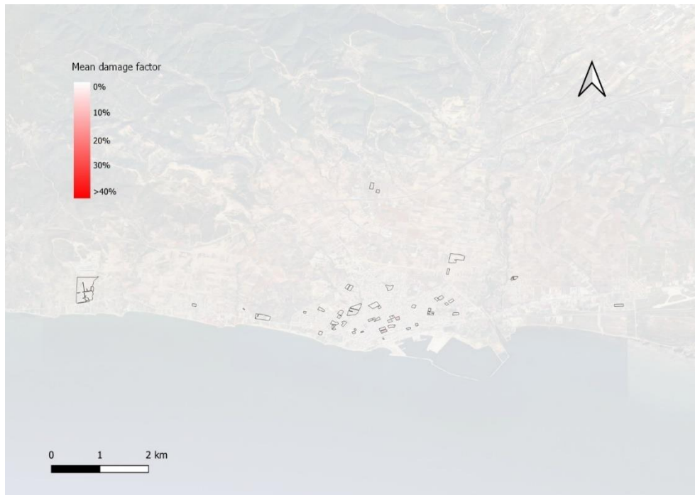
Figure 63. Spatial mean damage factor distribution for school buildings in Alexandroupolis for PSHA scenario with T_m=475 yrs.
