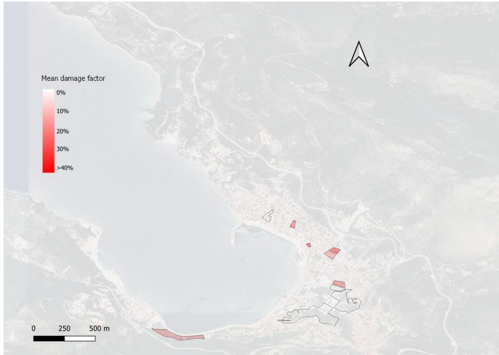
Figure 97. Spatial mean damage factor distribution for school buildings in Samos for the DSHA scenario of the Samos-North fault.
