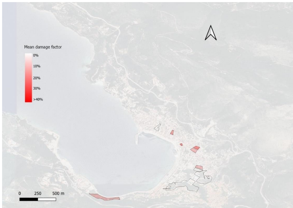
Figure 96. Spatial mean damage factor distribution for school buildings in Samos for PSHA scenario with T_m=950 yrs
