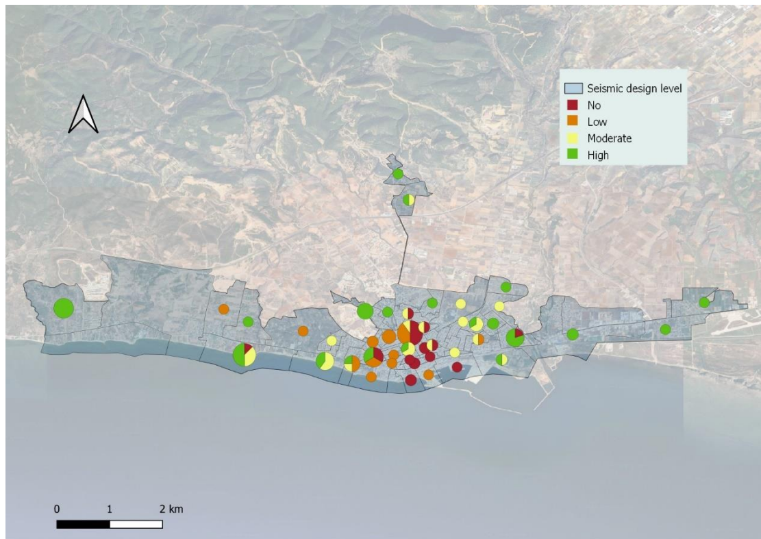
Figure 44. Spatial distribution of the seismic design level of school buildings in the city of Alexandroupolis (No: <1959, Low: 1960–1984, Moderate: 1985–1995, High: >1996)
